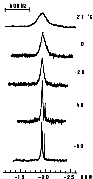
Fig. 3. Variable temperature ^1\text{H} NMR spectra of \text{HRuCo}_3(\text{CO})_{12} (7).
